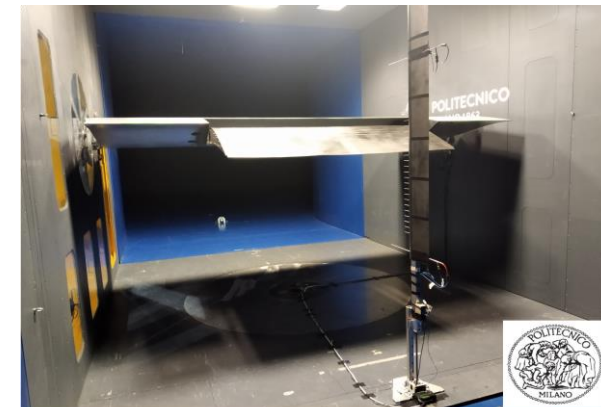
Large-Scale A320 SMS prototype (near scale 1) in the wind tunnel of POLIMI
